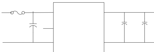
Figure 2. Typical Application of QTS48T25120
